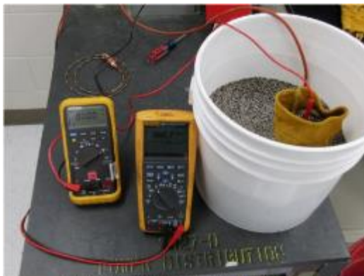
Figure 29 Testing a glove in metal shot
