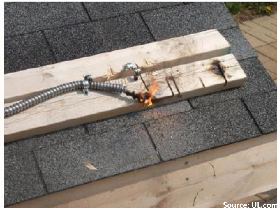
Figure 59 Open flame from arcing
