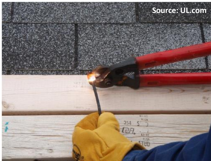
Figure 51 Cutting wire with cable cutter
