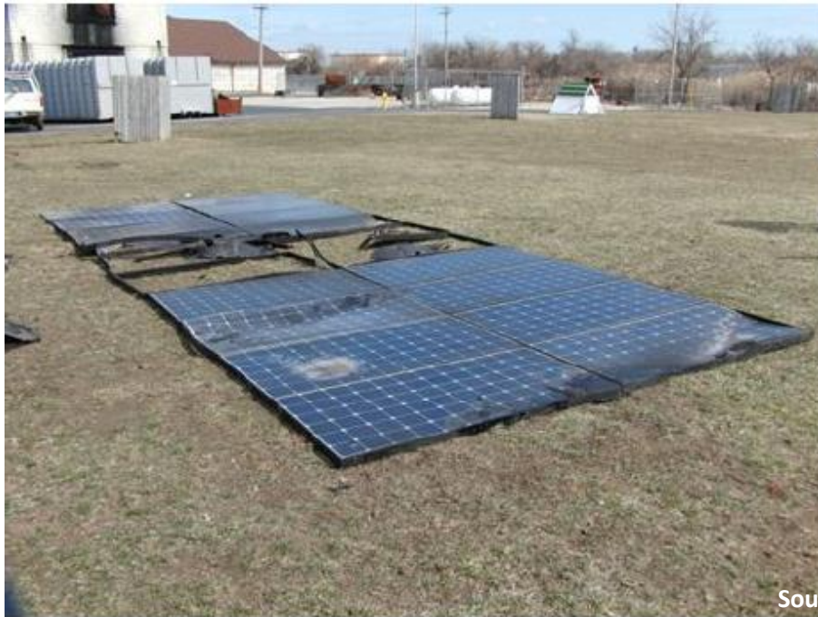
Figure 113 Post fire, front surface
