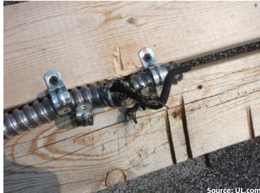
Figure 60 Exposed conductor from action of chain cutting
