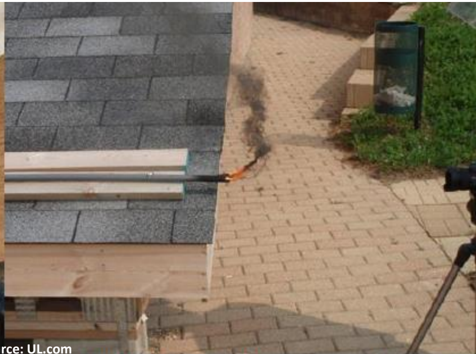
Figure 55 Open flame from arcing
