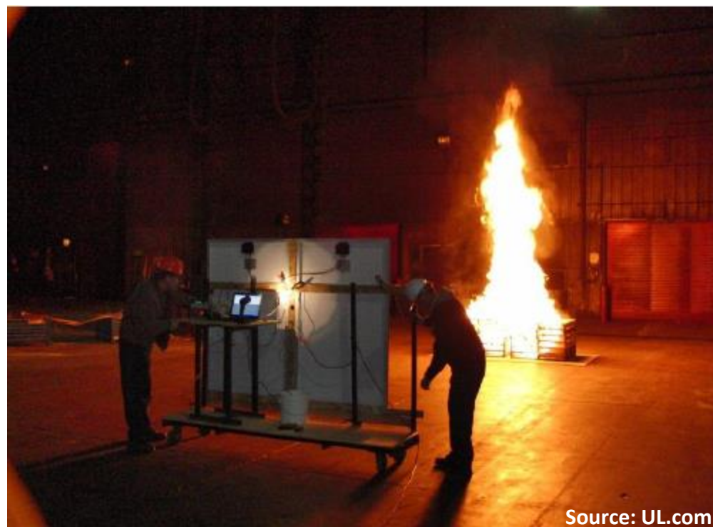
Figure 73 Test fixture with modules approaching fire
