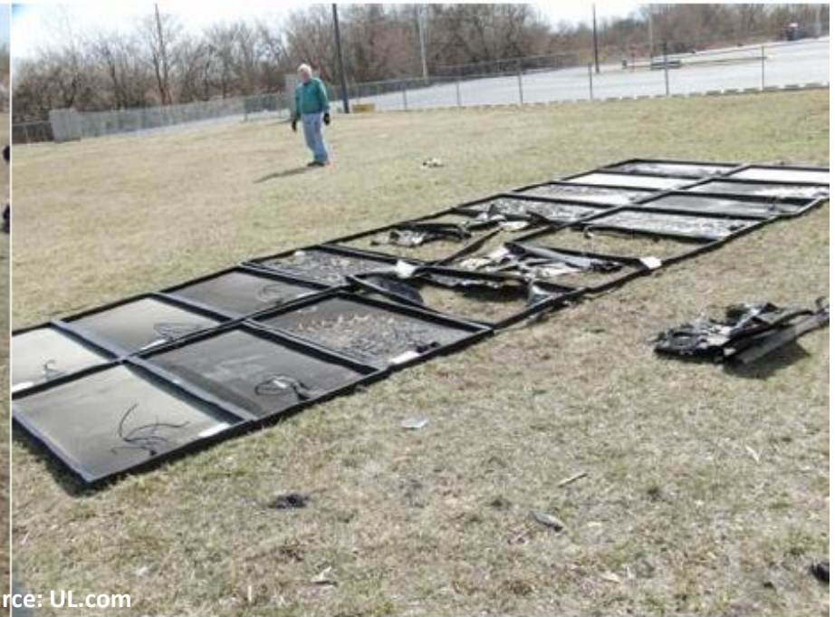
Figure 114 Post fire, back surface
