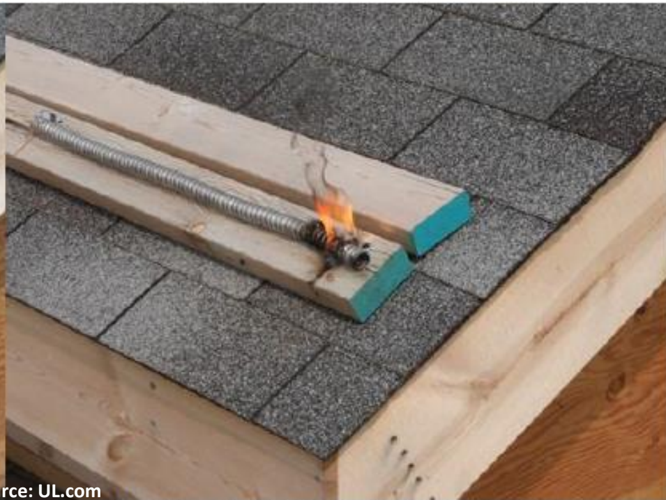
Figure 57 Open flame from arcing
