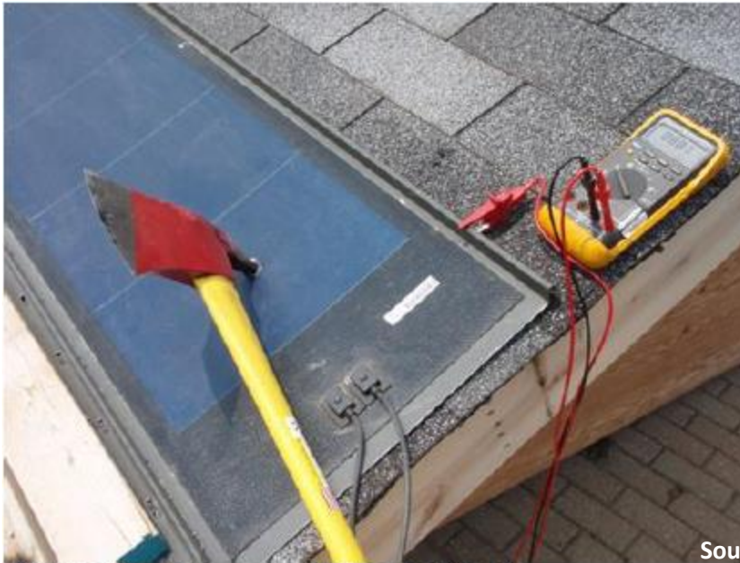
Figure 65 Axe penetrates laminate
