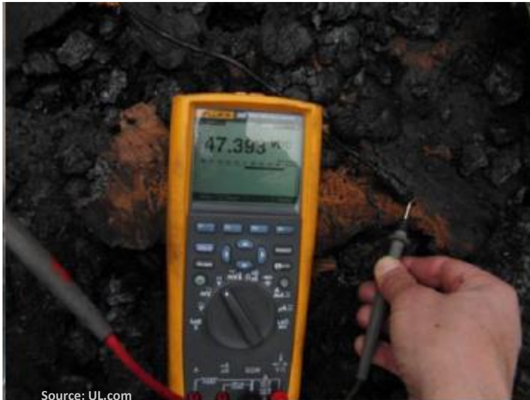
Figure 157 Voltage between exposed wires
